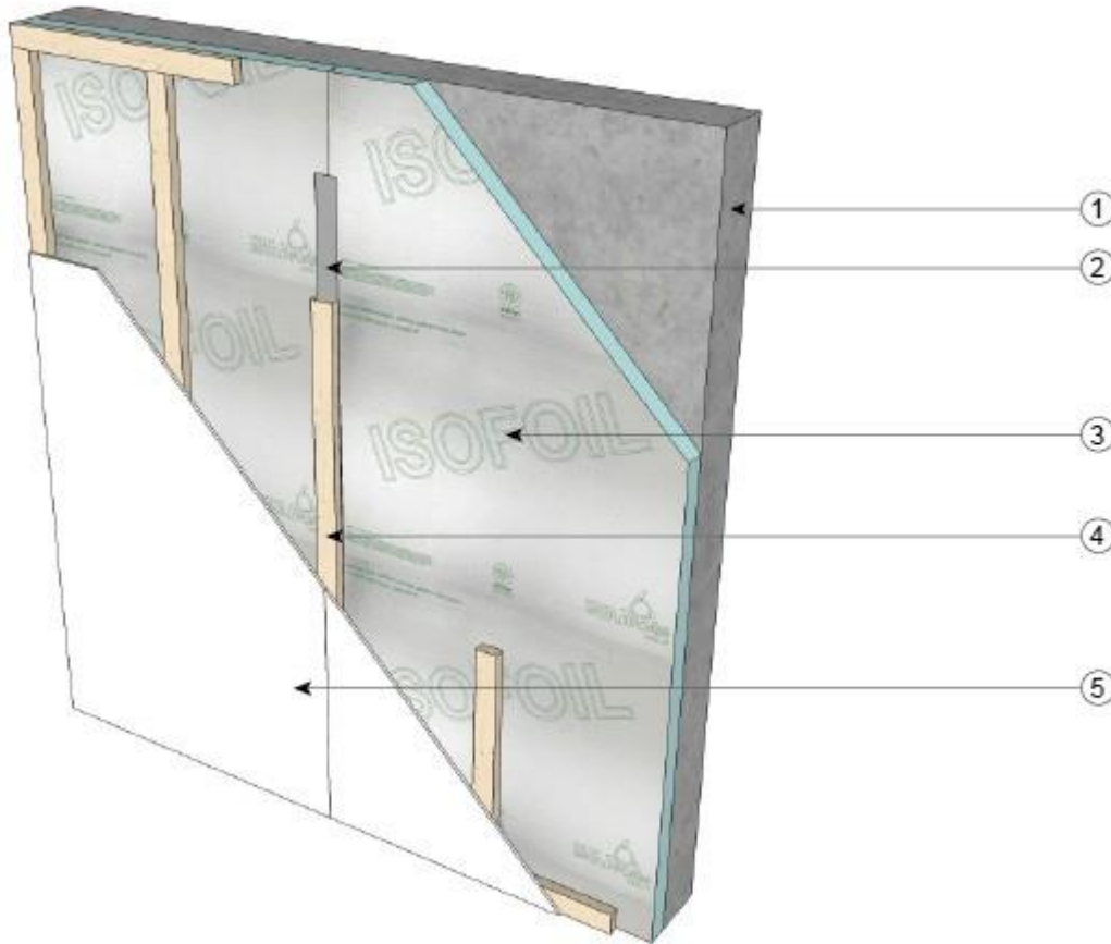
Figure 4. “Isofoil, PROfoil, EZfoil” adjacent to the furred air space assembly installed within the manufacturer’s designated wall assembly No. 4:
