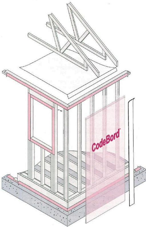
Figure 3. FOAMULAR® CodeBord® Air Barrier System (CABS) – Hybrid CABS with exterior seam and flashing tape
