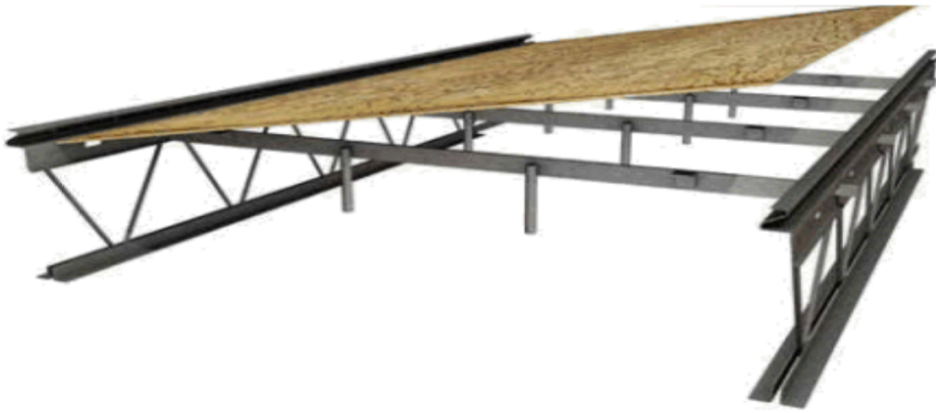
Figure 3. Hambro D500 open-web joist with temporary plywood deck
