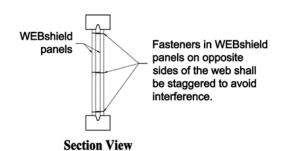
FIGURE C.1 - WEBshield Installation Details
